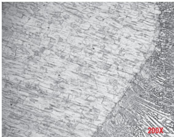
Fig. 8: HAZ of laser sample
