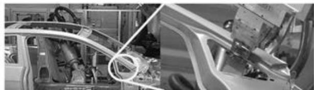
Fig. 1: Car body of Volkswagen Golf VII. Triangle window is welded with LaserSeamStepper
