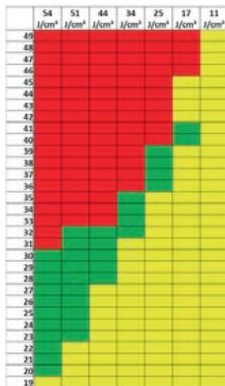
Figure 2: Summary of the delamination experiments (yellow: no effect on the front side, green: delamination of the CIGS film, red: penetration of the stainless steel substrate).
