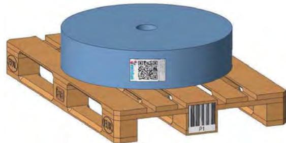
Figure 6. Roll of foil labeled by QR code and pallet labeled by Code 39.
