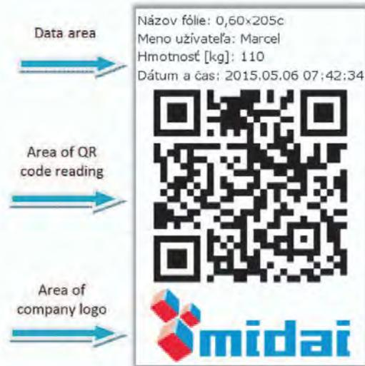
Figure 10. Designed pattern of the label with the code
