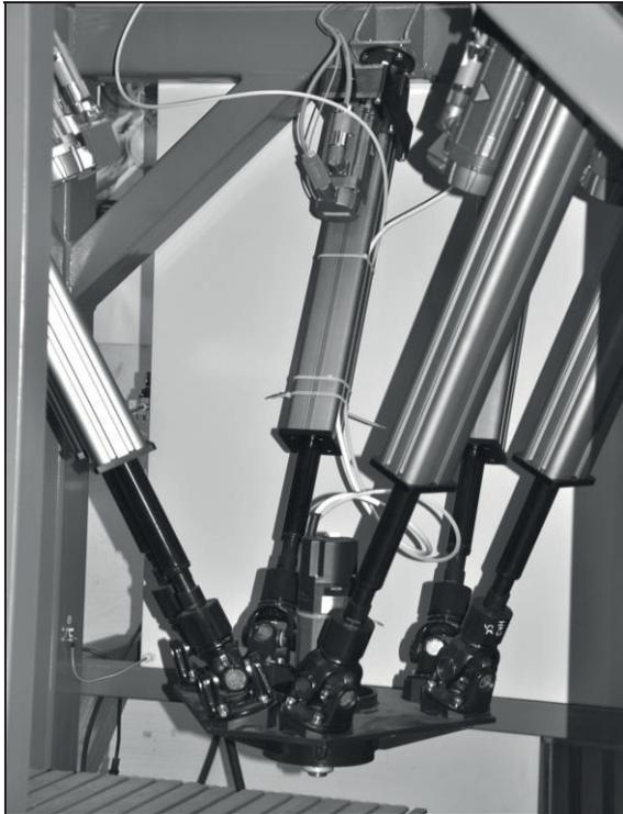
Figure 1. Hexapod prototype
