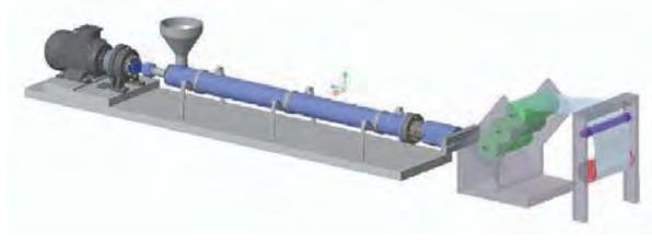
Figure 3. Extruder for foil production (length 17m).
