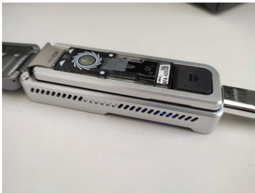
Figure 3: Flongle adapter attached to MinION sequencer from ONT for sequencing prepared DNA samples
