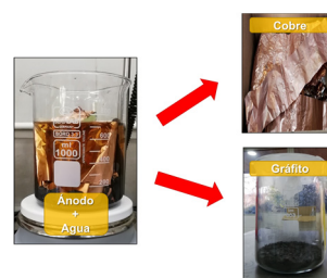
Fig. 4. Recovery of copper and graphite.
