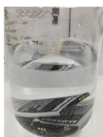
Fig. 2. Battery discharge in 1M NaCl solution.
