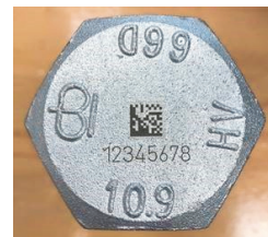
Fig. 2: QR Code engraved on bolt
