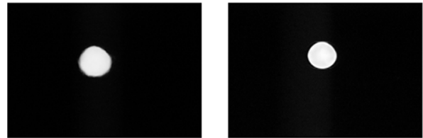
Fig. 15. Nickel, t=6 mm; Entry diameter 168µm (left); Exit diameter 148µm (right)
