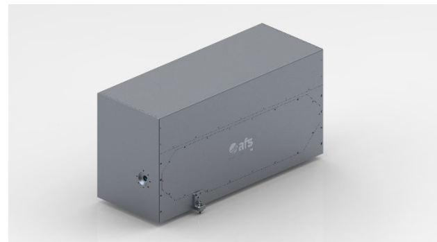
Figure 7: Rendered view of the second generation of our compact 2- \mu\text{m} laser featuring a volume of approx. 800 \times 300 \times 350\text{mm}^3 only.
