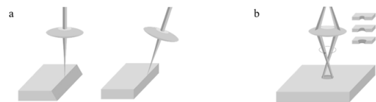
Fig. 4. (a) Influence of inclination angle on wall angle (schematic); (b) Tilted rotating laser beam allows drilling with positive and negative wall angle as well as cylindrical holes (schematic). [4]
