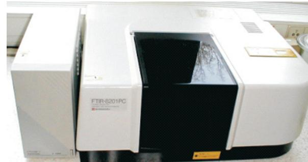
IR-Spectrometer SHIMADSU FTIR 800
