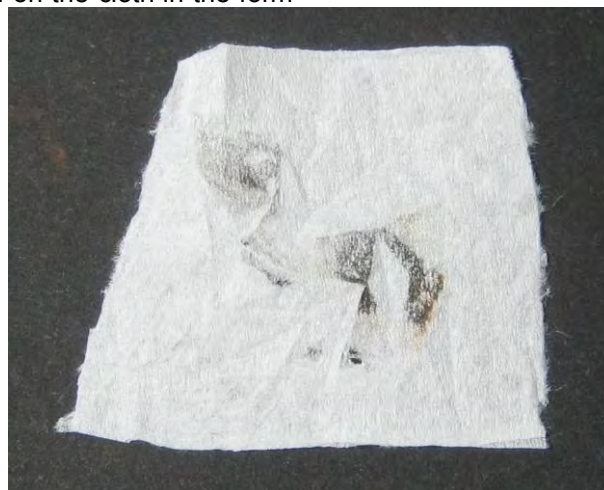
Figure 2 - Cloth used for rubbing off colors of laser marking after being held in a solution of salt in water.
