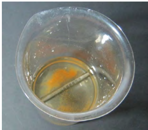
Figure 10 - Low-alloy steel that is laser marked placed in a solution of 20% salt water. In the vessel a clearly expressed residue can be seen.
