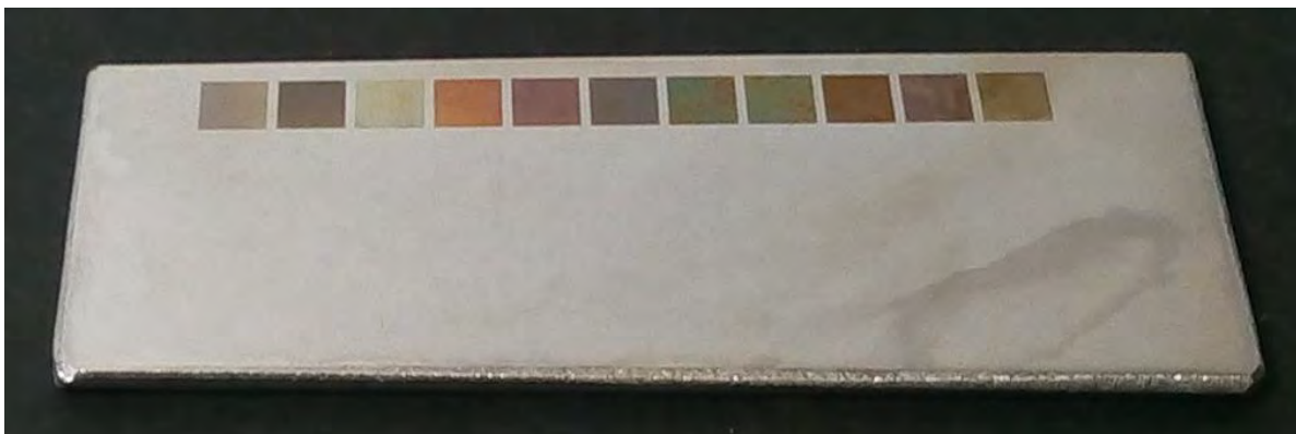
Figure 3 - The modified appearance of original 11 laser marking colors after being held in salt water solution.
