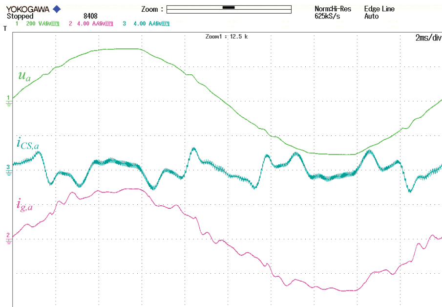
Figure 10: Selective harmonic compensation with voltage controlled APF
