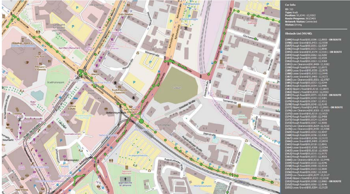
Figure 4: Our simulation visualizes vehicular ad-hoc networks in realistic urban environments using OpenStreetMap material. Information about obstacles is shared either globally or locally with every new encounter. Each data package is traceable and our visualization provides an overview of the data currently available to selected vehicles (gray panel on the right).
