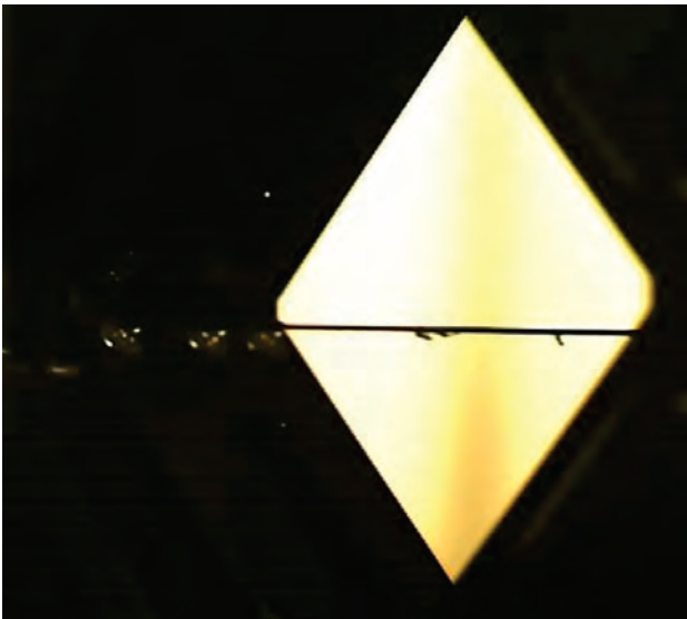
Fig. 2 Excessive material stuck on coated wire. Shot taken from high speed camera
